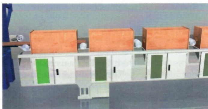
Figure 3: Production Start Sequence: Cold bar entering the furnace from the left (green panel indicates energized furnace zone). Each zone is automatically turned on as the bar enters.
