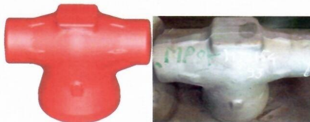
Figure 5 - Simulation and actual result correlation
