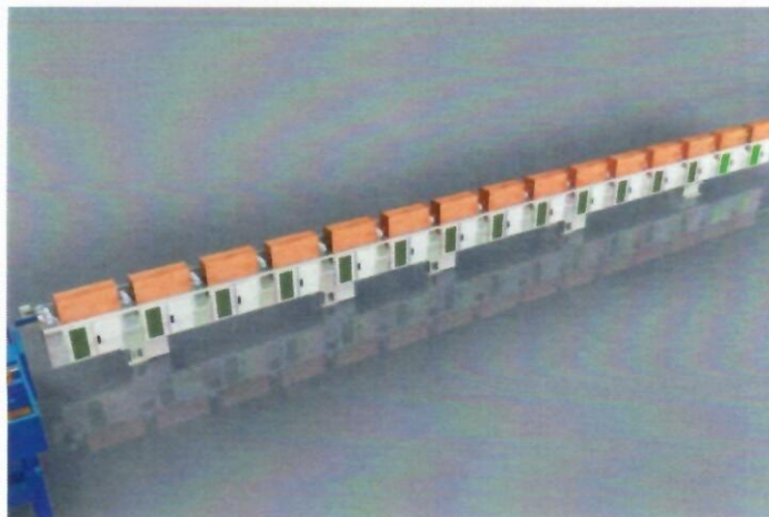
Figure 4: Production Stop Sequence with final bar exiting the furnace (green panels indicate energized furnace zones). Each zone is automatically turned off as the bar exits.
