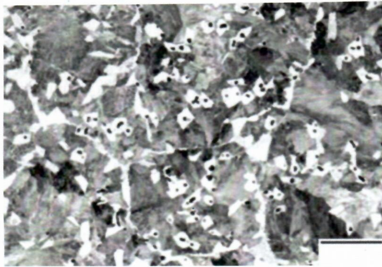
Figure 2. The microstructure of a medium-carbon vanadium micro alloyed steel. The addition of vanadium allows the ferrite (white) phase to form on the MnS particles (black bull's eyes in the ferrite) and break up the large pearlite (black) colonies in the microstructure.
