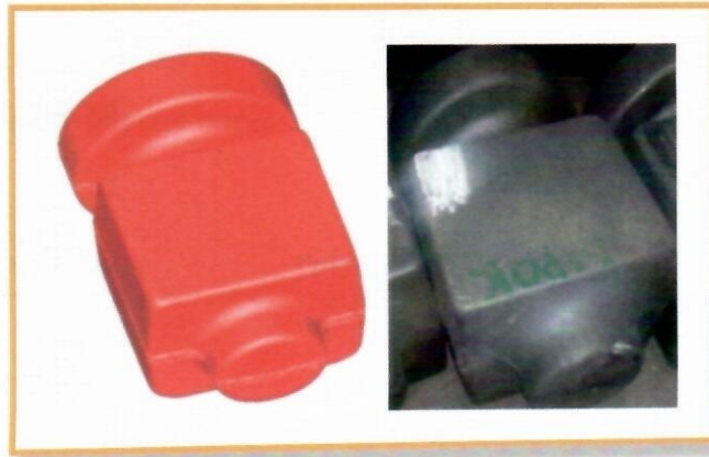
Figure 12 - Comparison of simulated component and actual forged component
