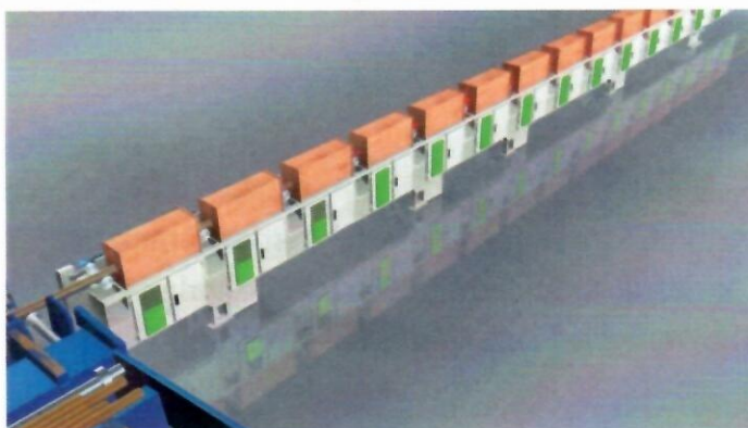
Figure 7: Soft Heating of Crack-Prone Steels (Green panel indicates energized furnace zone.) Zones one through three provide soft heating below the curie temperature to prevent thermal cracking, without using special soft heating coils.
