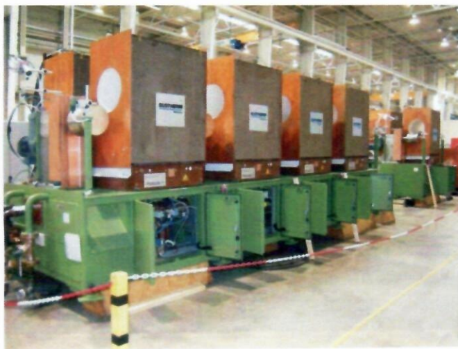
Figure 2: High performance induction furnace for large bar heating
