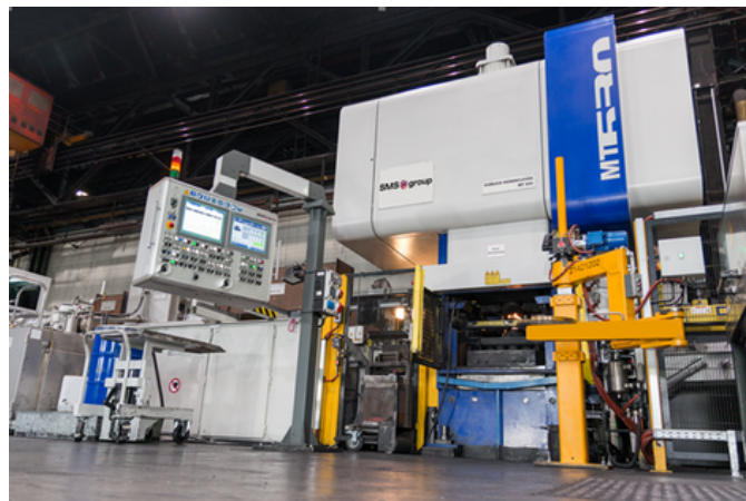
Caption: The first MT 630 eccentric press with MEERTorque® drive unit at SONA BLW Präzisionsschmiede GmbH, Germany
