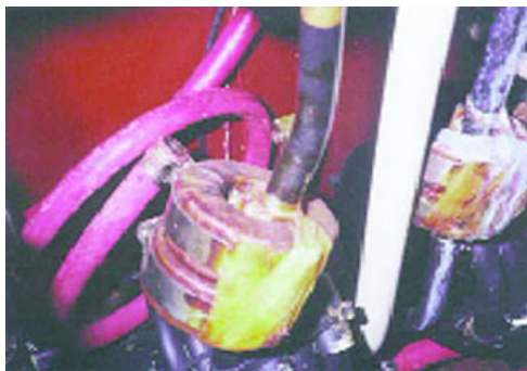
Electrolysis causes erosion, resulting in a hose leak failure
